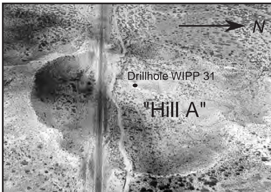
Figure 6. Aerial photograph of the surface collapsed dome structure of "Hill A," one of the breccia pipes over the Capitan reef in the northern end of the Delaware Basin. Bachman (1980) and Snyder and Gard (1982) showed the relationship to the Capitan and that the doming is caused by lowering of the surrounding area by dissolution of upper Salado salt after collapse.
